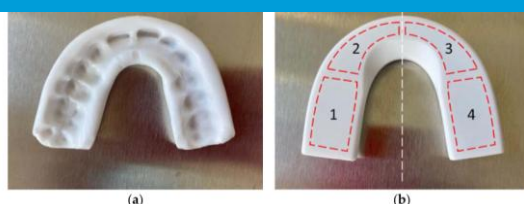
Figure 2: Force-sensing oral appliance. (a) Top view showing the maxillary arch impression. (b) Occlusal plane view with four embedded pressure sensors. Courtesy of Maoddi P. et al. 11
