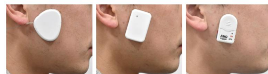
Figure 1: Ultra-miniature portable electromyographic devices used for bruxism detection. Courtesy of Mikami S. et al. 10
